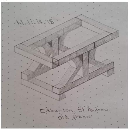
Today, they are fixed between two parallel wooden Beams. 1.A in the Pickford scheme.
